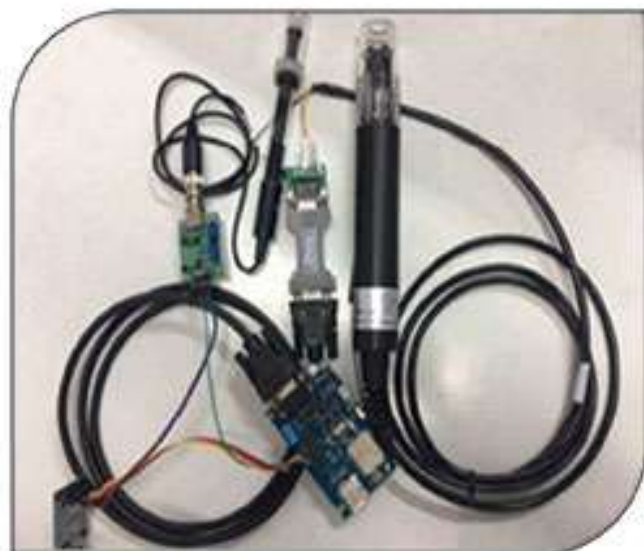
Fig. 4. Sensor measuring DO, Temp, pH (Source- Huan et al., 2020)
